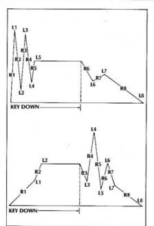
Fig. 1. Two possible CZ envelopes, showing rate and level settings. Level 5 is the sustain level in the first envelope, while level 2 is the sustain level in the second envelope.
